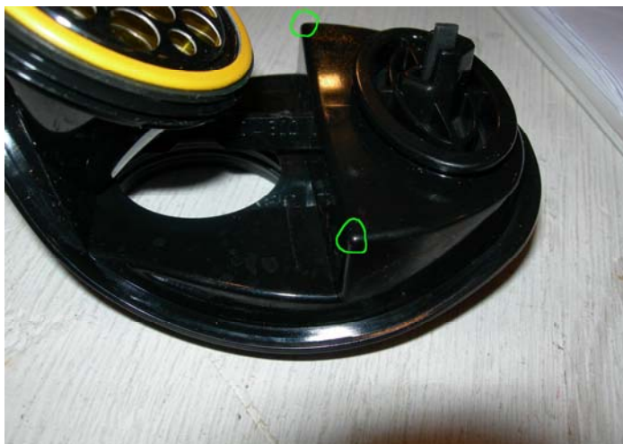
Location of where pinholes have formed (green circles).
