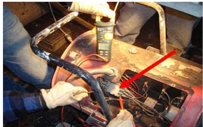
Photo 2 - Electrical contacts that prevent overheating.
