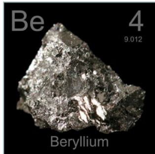
Figure 1-1. This pure broken crystal of refined beryllium ordinarily would be melted down and turned into strong, lightweight parts for missiles and spacecraft
