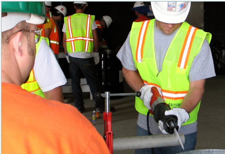
Figure 1-2. New worker being coached by trainer (in orange) on safe use of reciprocating saw
