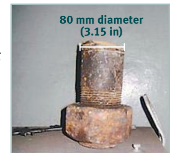
Figure 1-2. Degraded bolt found post-accident
