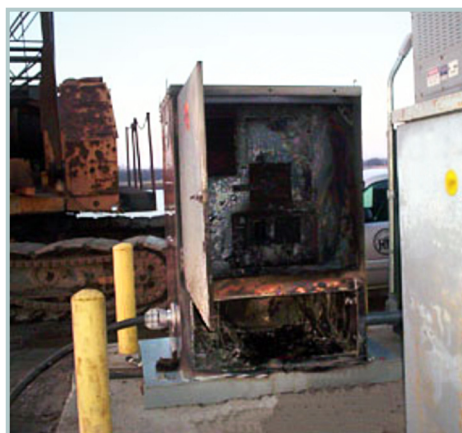
Figure 1-3. Damage to electrical cabinet in fatal Iowa accident
