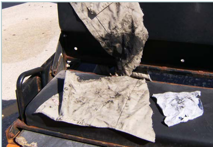
Figure 1-2. Grease mark from trailer on injured worker's shirt (cut from worker post-accident)
