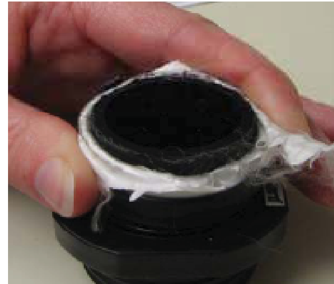
Figure 1-2. The rough and sharp edge can be seen around the edge of the black tube (fitting)
