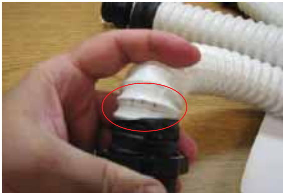
Figure 1-1. Small holes in white plastic breathing air tube (red circle)
