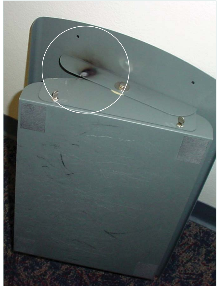
Figure 2-1. Burn mark at top of footrest
