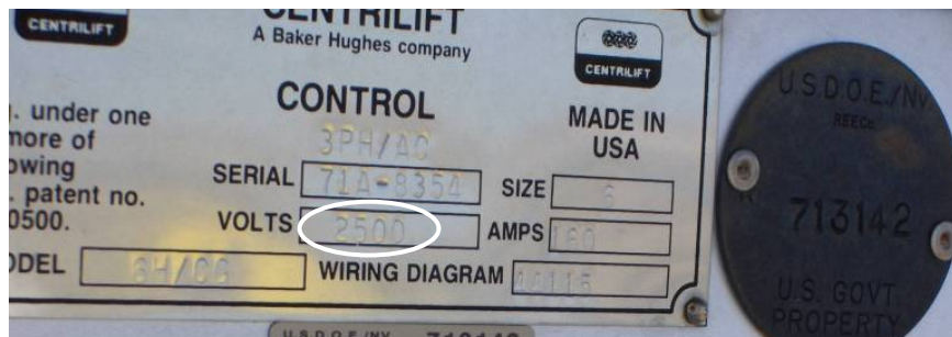
Figure 1-3. Manufacturer's nameplate showing "2500" in the volts block (circled)
