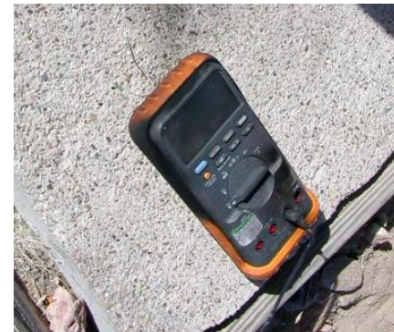
Figure 1-2. Closeup of the damaged multimeter
