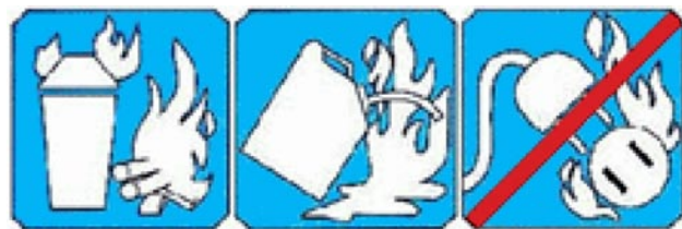
Figure 1-3. Label showing fire extinguisher NOT suitable for electrical fire
