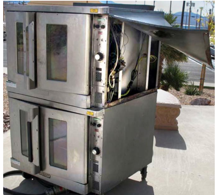
Figure 1-1. Oven after fire in back panel
