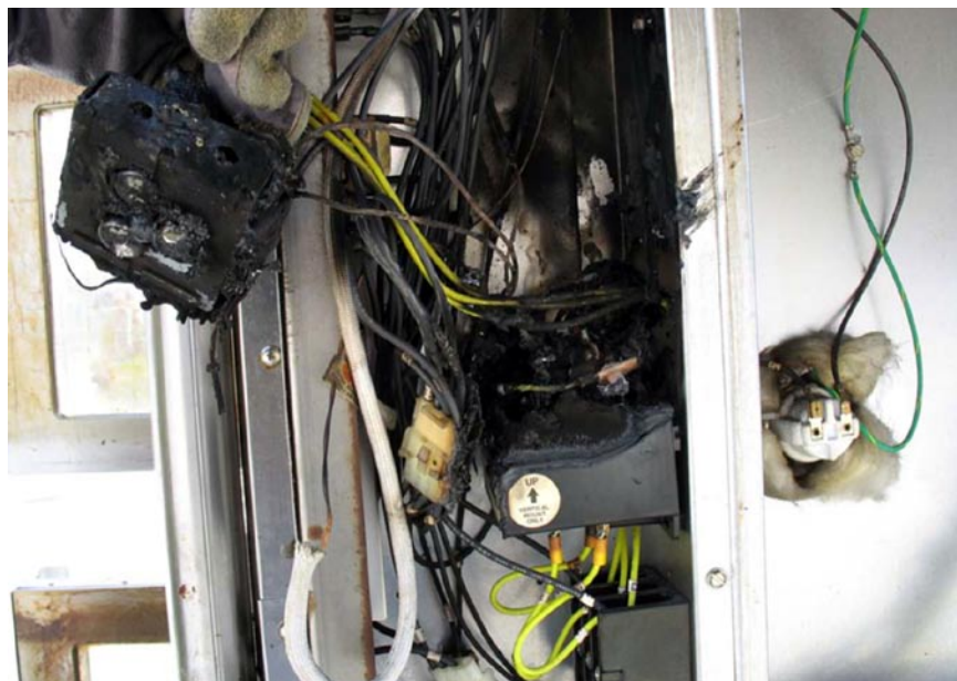
Figure 1-2. Electrical controller housing involved in the fire
