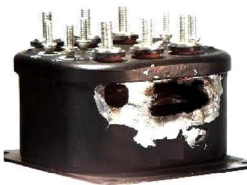
Figure 3-3. Damage from metal vapor arc
