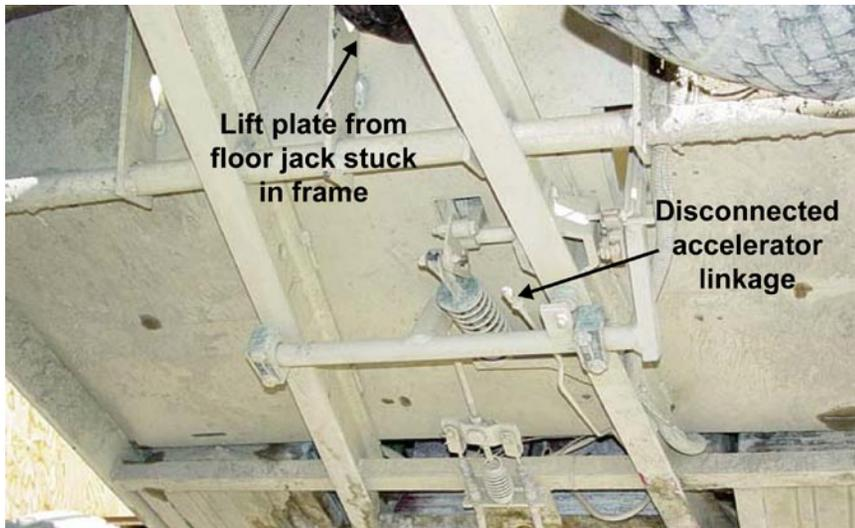
Figure 1-3. Cart undercarriage (note disconnected linkage and lift plate)
