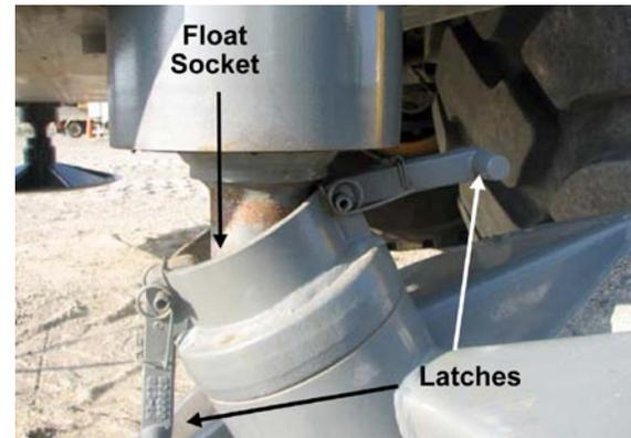
**Figure 2-2. Quick-release float showing latches**
