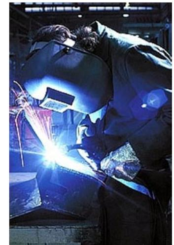
**Figure 3-3. Welding can produce hexavalent chromium**
