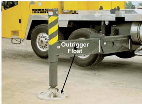
**Figure 2-1. Outrigger and float shown deployed**
