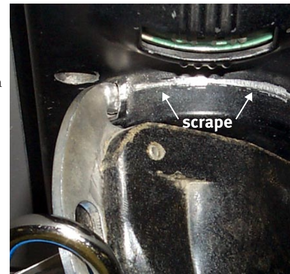
Figure 2-3. Close up of locking device
