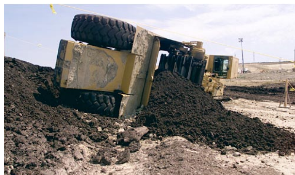
Figure 3-1. Scraper following rollover
