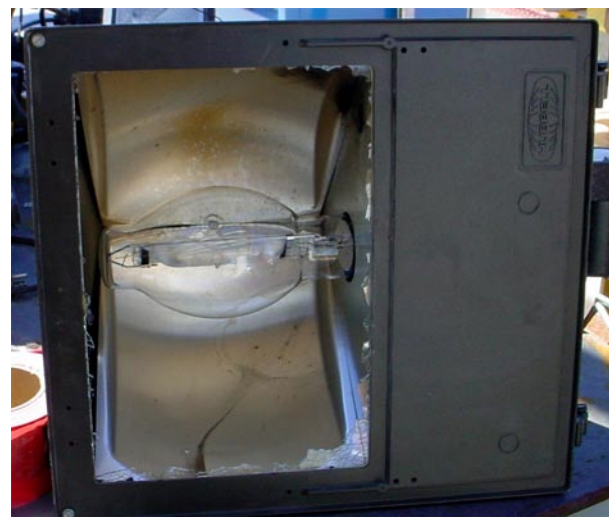
Figure 2-3. Floodlight with broken lens
