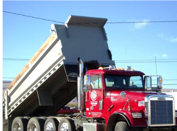
Figure 1-1. Raised bed in contact with power line
