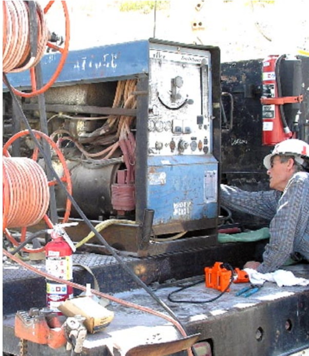
Figure 2-1. Welder/generator (blue) on bed of mechanic truck
