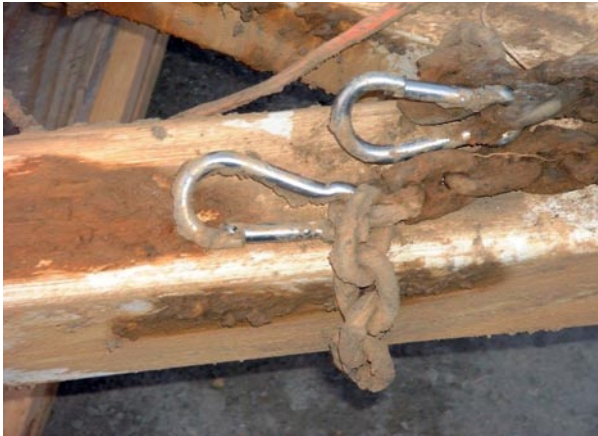
Figure 3-3. Post-accident photo showing unattached safety chains
