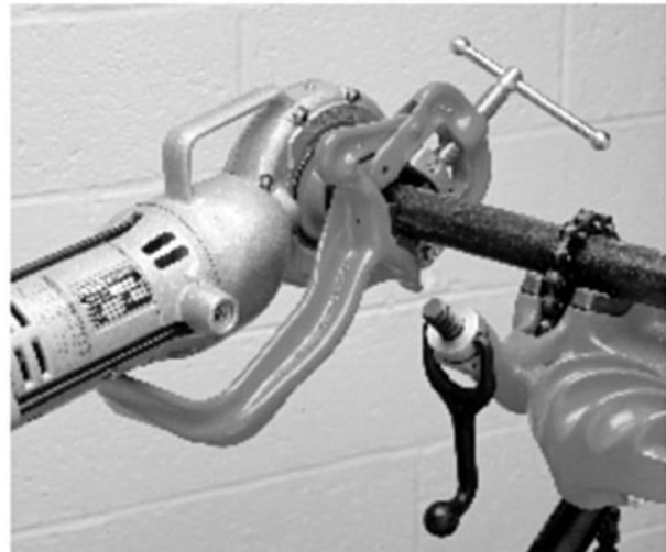
Figure 1-2. Recommended support arm
