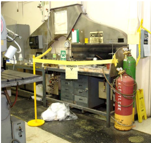
Figure 2-1. Contaminated work area and the gas bottles for the torch used to heat the collimator
