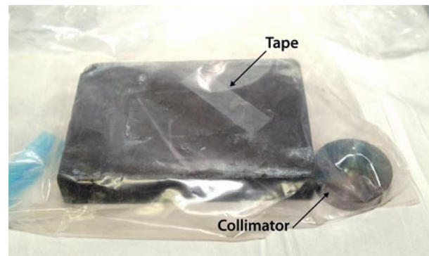
Figure 2-2. Graphite block with tape to fix the cobalt-57 powder and the collimator that held the source
