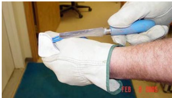
Figure 1-2. How the worker used the sharpener
