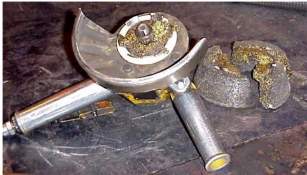
Figure 2-3. Damaged grinder and cup stone
