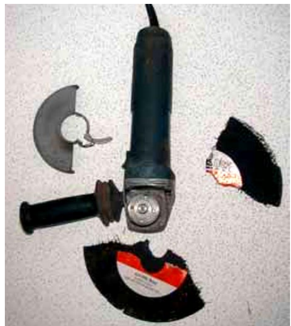
Figure 2-1. Disintegrated grinding wheel
