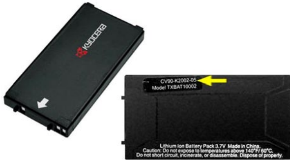
Figure 4-1. An identified defective Smartphone battery
