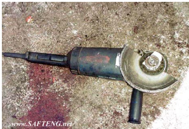
Figure 2-2. Grinder missing the disk
