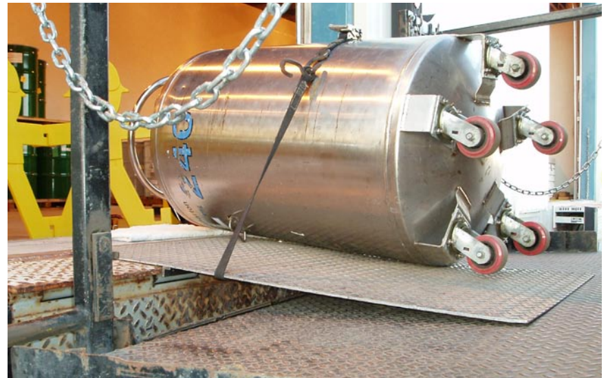
Figure 2-2. Dewar strapped to truck rail and ramp
