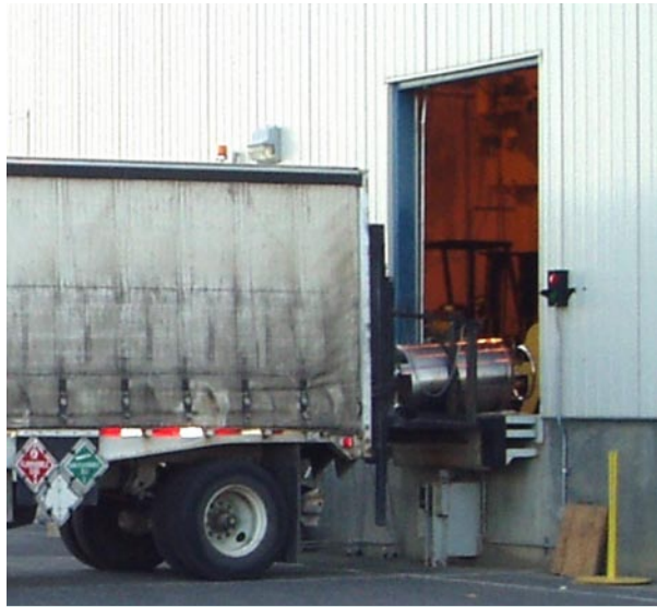
Figure 2-1. Truck at loading dock with fallen Dewar
