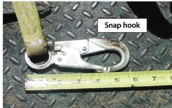
*Figure 3-2. Lanyard snap hook showing burn marks*
