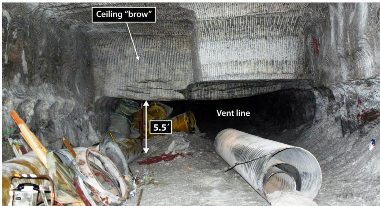
**Figure 2-1. Vent pipe in the drift**
