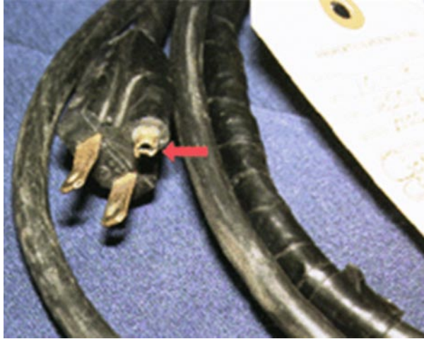
Figure 4-1. Worn cord and damaged grounding prong
