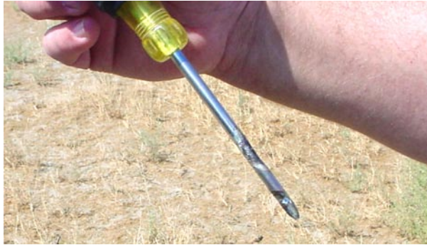
Figure 2-1. Burned and damaged screwdriver
