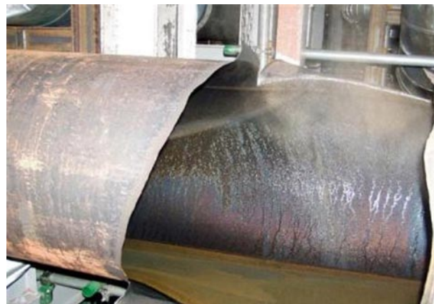
Figure 1-3. Close-up of pipe break
