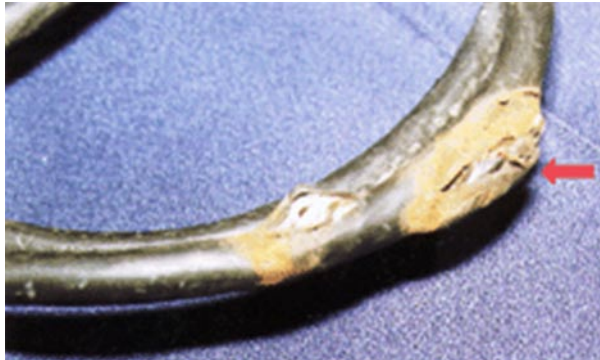
Figure 4-2. Cord with damaged insulation
