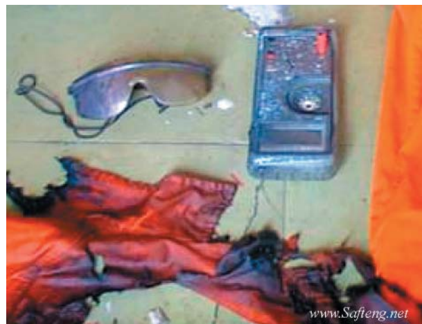
Figure 4-1. Accident victim's clothing, destroyed digital multimeter, and damaged safety glasses
