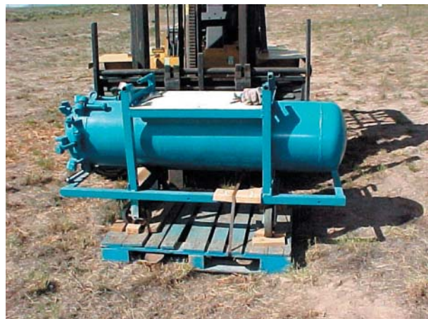
Figure 4-1. Overpack containing the leaking cylinder
