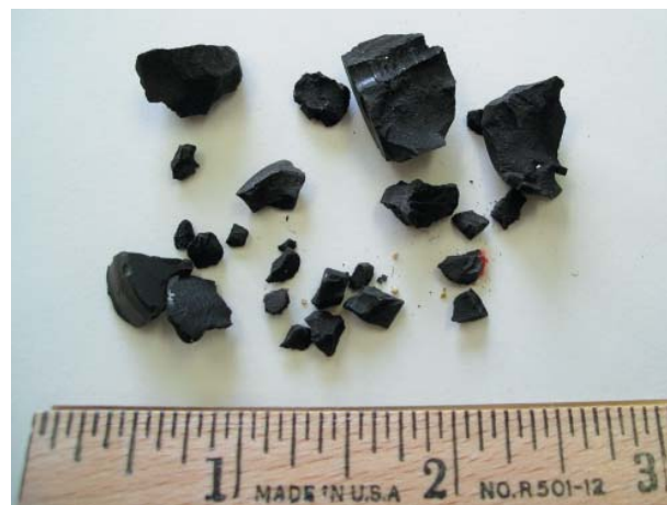
Figure 1-3. Debris expelled from inside electrical connection on squib
