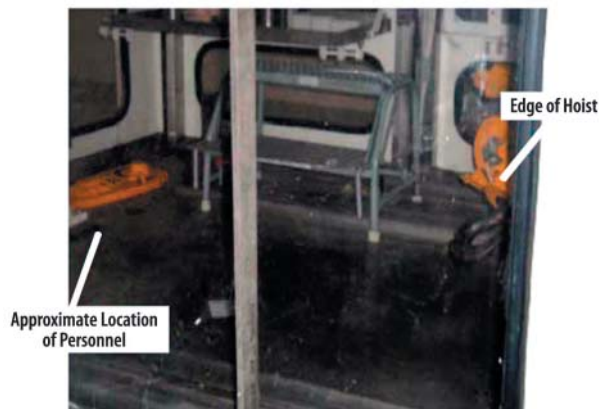
Figure 3-1. Location of hoist following dropped load
