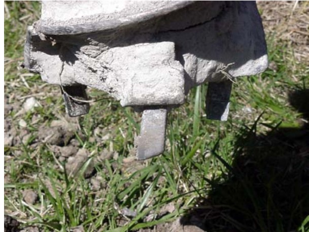
Figure 2-1. Concrete on drill bit
