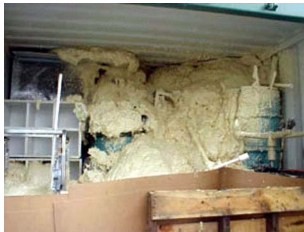
Figure 4-1. Autofroth in a waste cargo container
