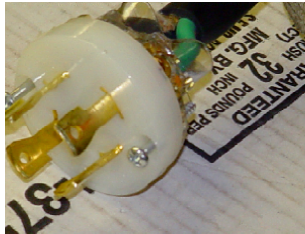
Figure 1-2. The miswired plug
