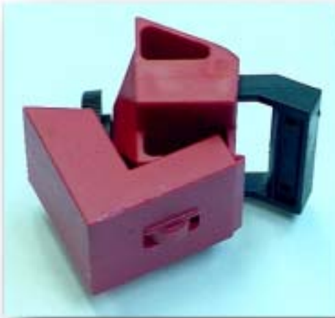
Figure 5-1. Locking device that fell off the circuit breaker handle
