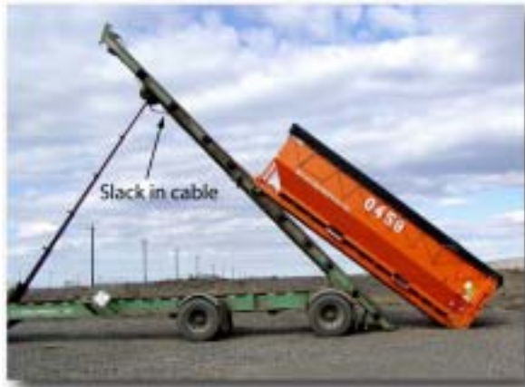
Figure 2-3. The investigators introduced slack in the hoisting cable
