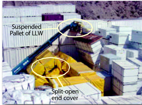
Figure 4-2. Accident scene following stack collapse
