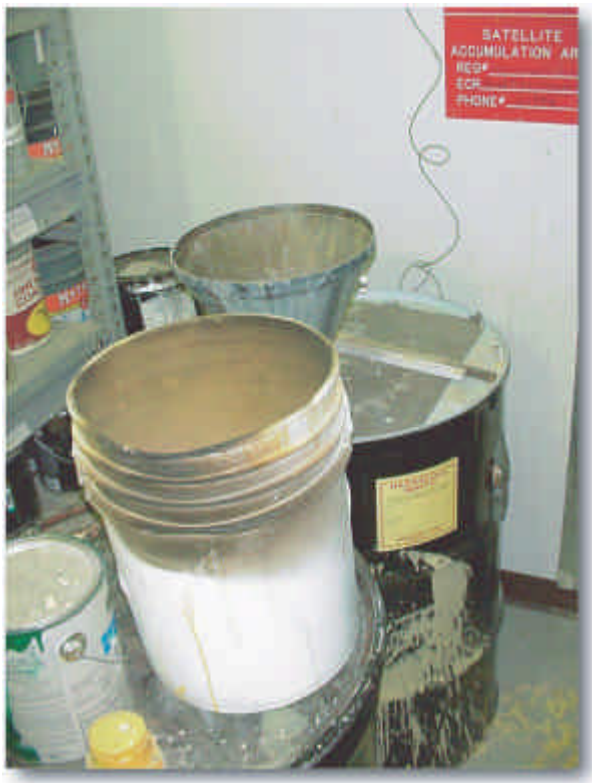
Figure 2-1. The solvent drum and plastic bucket involved in the fire
