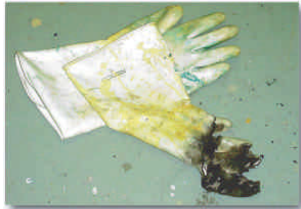
Figure 2-2. The burned gloves
