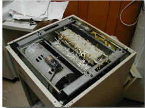
Figure 3-2. The shredder after the fire
