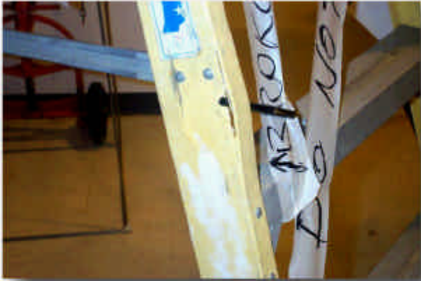
Figure 4-2. Cracks in the ladder's leg
