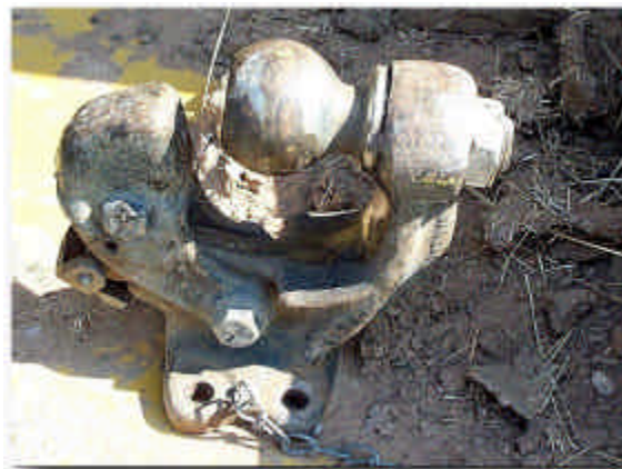
Figure 1-2. Trailer hitch after detachment from truck
