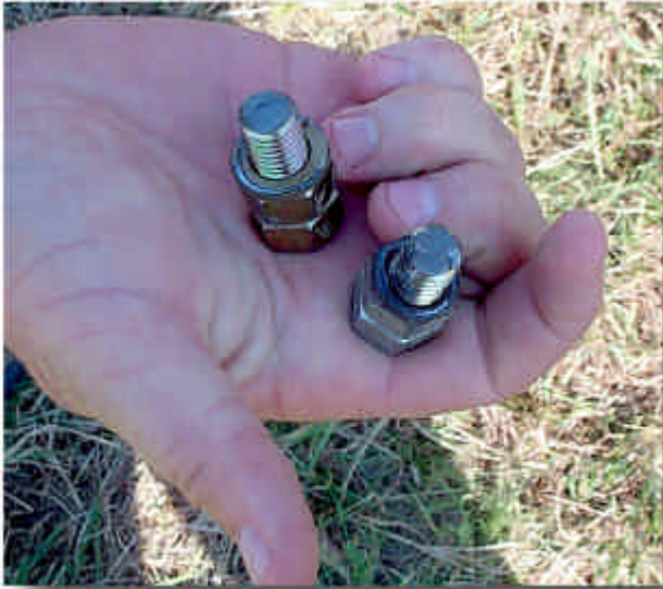
Figure 1-3. Two of the four sheared trailer hitch bolts
