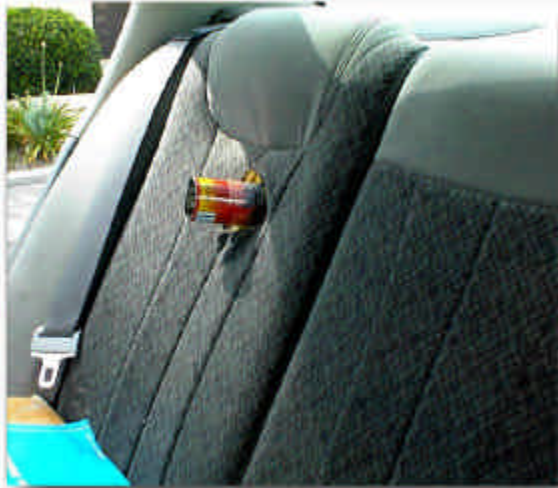
Figure 3-1. Exploded aerosol can embedded in rear seat
