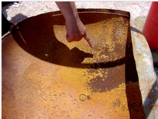
Figure 4-4. Acid corrosion inside the cylinder
