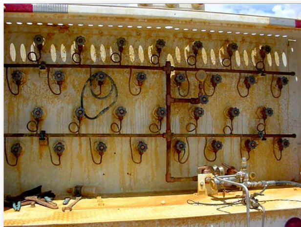
Figure 4-3. Acid spray on nearby equipment
