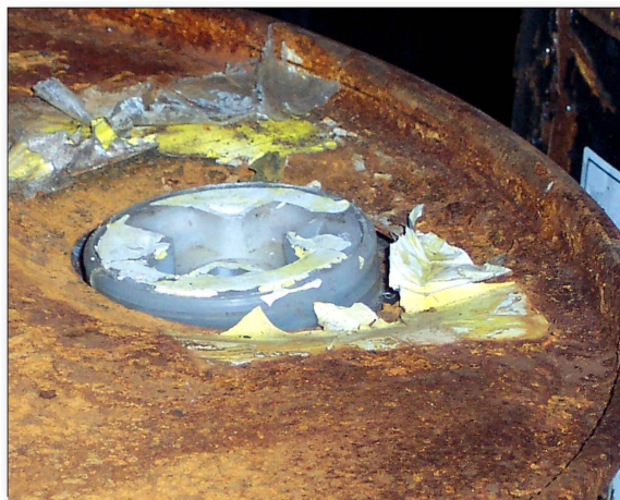
Figure 3-2. Degraded bung on waste drum
