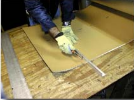
Figure 4-2. Scoring the aluminum wrap with a safer straightedge
