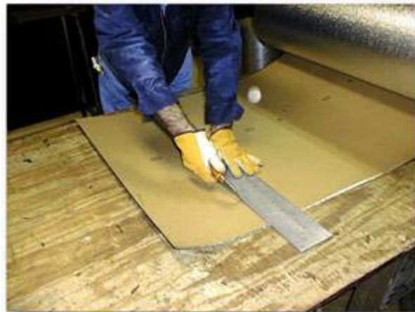
Figure 4-1. Scoring a straight line on aluminum wrap with a simple straightedge
