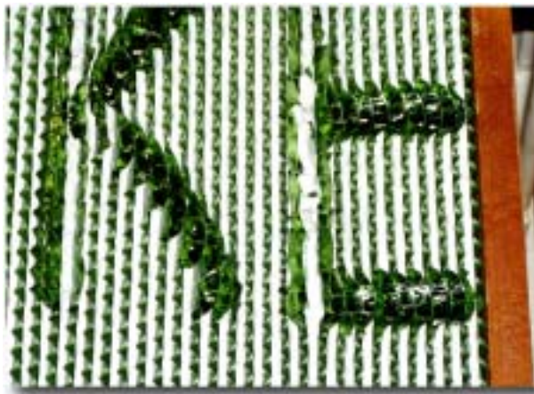
Figure 3-2. Another HEPA filter showing damage
