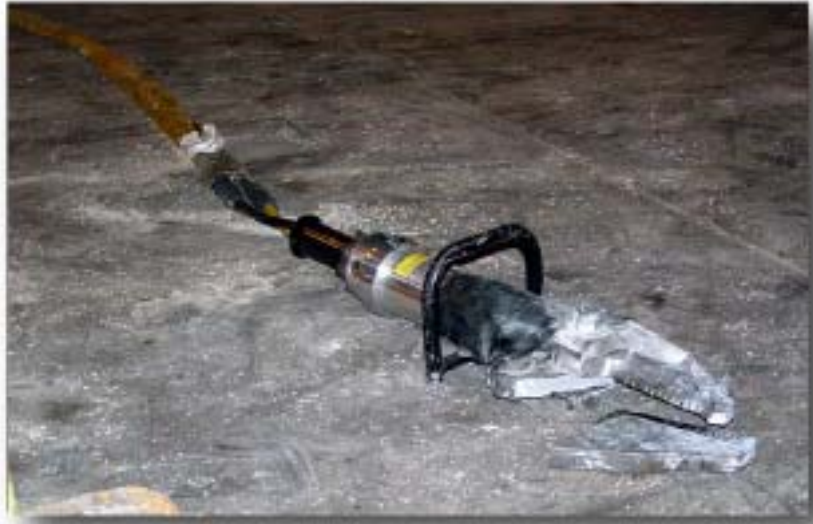
Figure 5-2. The broken shear and blade fragment
