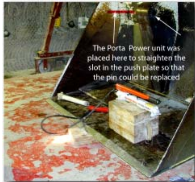
Figure 4-1. The location on the bucket where the Porta Power was used
