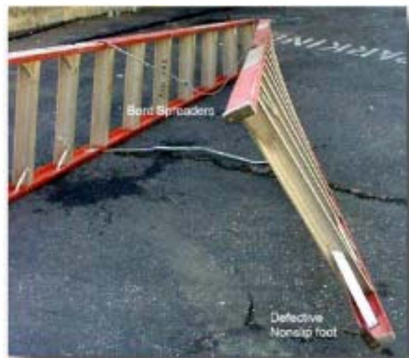
Figure 2-2. The damaged ladder
