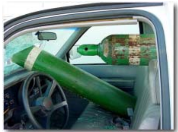
Figure 5-1. The cylinders shifted in the truck bed
