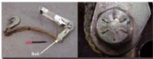
Figure 3-4. Ratchet tie-down strap and suspect/counterfeit bolt
