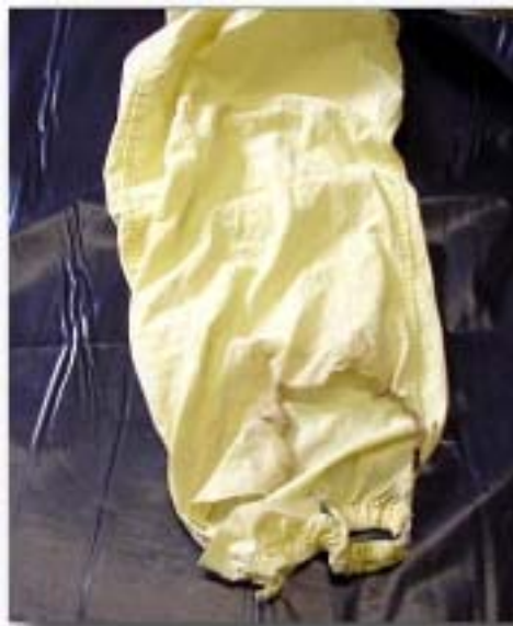
Figure 4-2. Scorched leg of PPE
