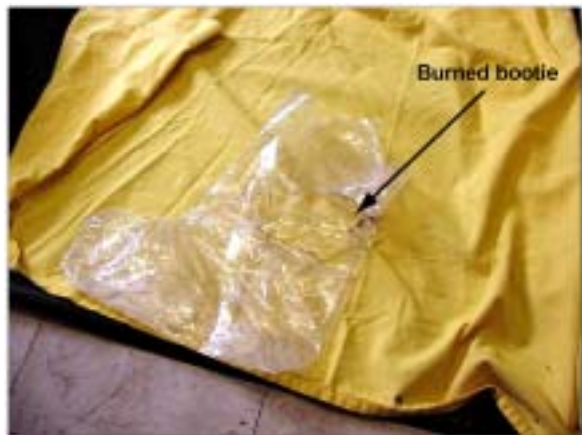
Figure 4-1. Worker's PPE and bootie
