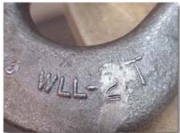
Figure 3-5. Tampering on a swaged lifting sling hook
