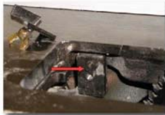
Figure 1-3. Mounting channel and through-pin (red arrow)
