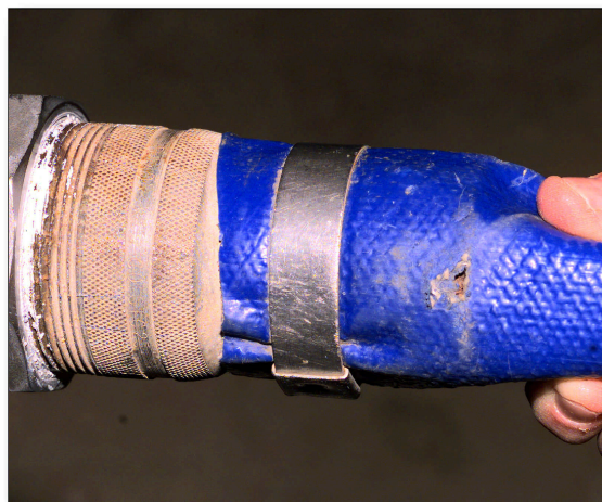
Figure 3-2. Defective fire hose
