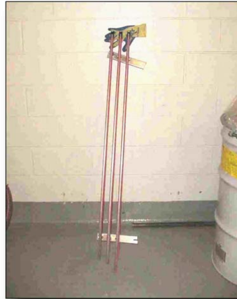
Figure 3-2. Section of buss bar that fell
