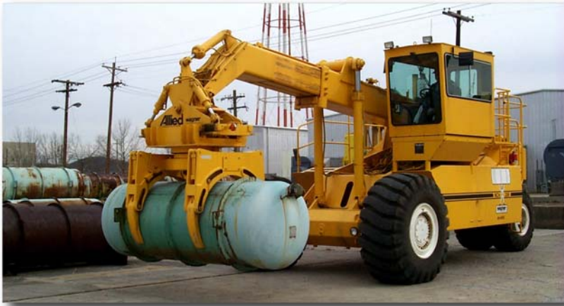
Figure 3-1. Allied-Wagner cylinder handler
