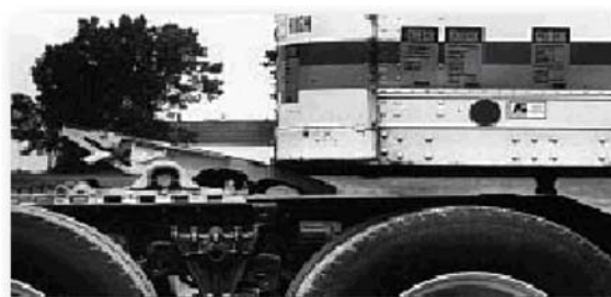
Figure 2-1. Uncoupled tractor and trailer
