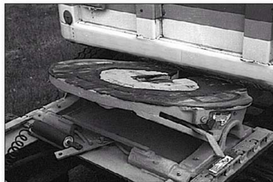
Figure 2-3. Lower fifth-wheel plate
