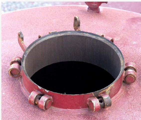
Figure 3-4. Pot opening and six threaded steel hold-down blocks
