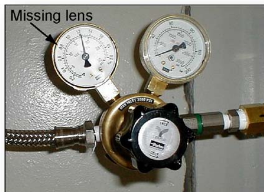
Figure 4-2. Damaged regulator (picture rotated 90 degrees)
