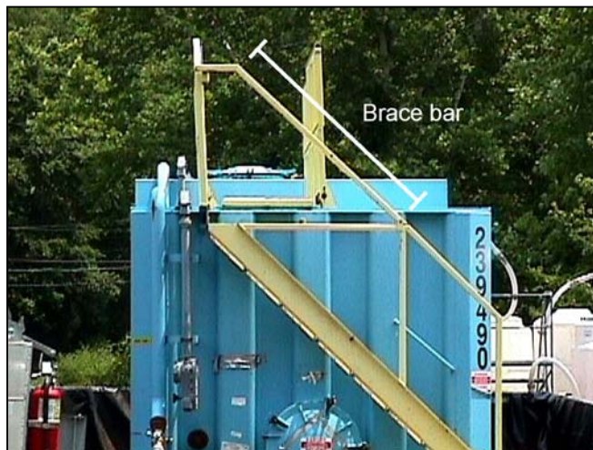
Figure 3-2. The worker was attempting to attach the brace bar to the handrail when he fell
