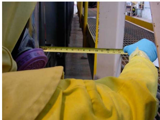
Figure 2. The clearance space between the railcar and the platform
