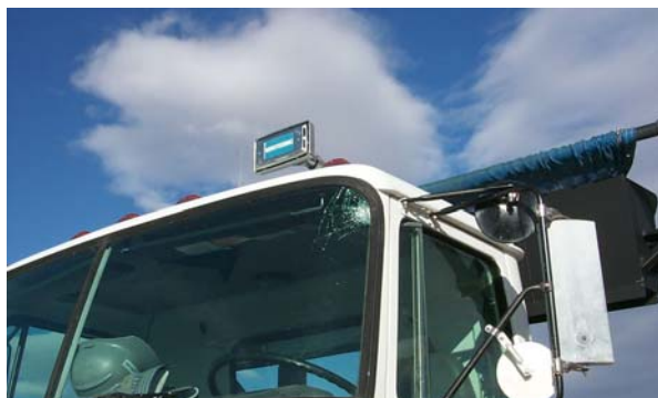
Figure 2. The cracked windshield
